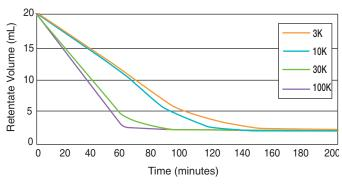
Protein solutions were processed in each of the Macrosep Advance devices. Average time (minutes) is plotted against mL of remaining product to be filtered using a swinging bucket rotor at 5,000 g. Solutions are 3K: Protamine Sulfate, 0.1% in 1X PBS; 10K: Cytochrome C, 0.025% in 1X PBS; 30K: IgG, 0.1% in 1X PBS; and 100K: Apoferitin, 0.1% in 1X PBS.
